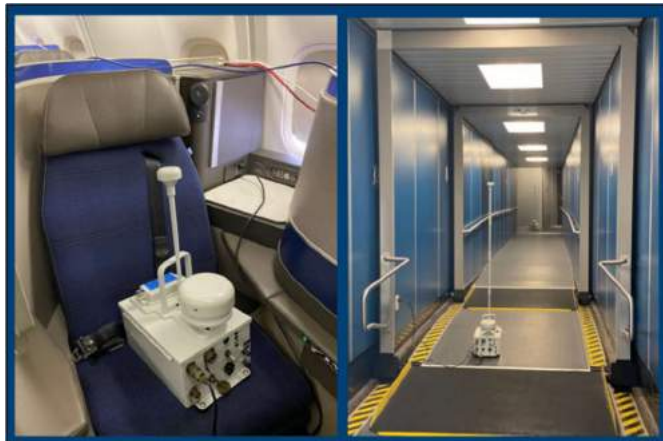
Figure 6. 777-200 Terminal/Jetway MID-AFT tests
